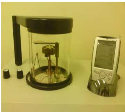
Figura 4 - Evaporadora (Sputter) Denton Vacuum - Desk III R.
