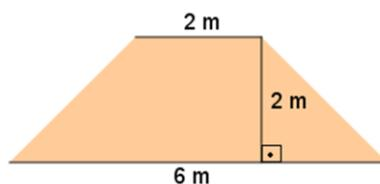
$$A = \frac{(B+b).h}{2} = \frac{(6\text{ m}+2\text{ m}).2\text{ m}}{2} = 8\text{ m}^2$$
