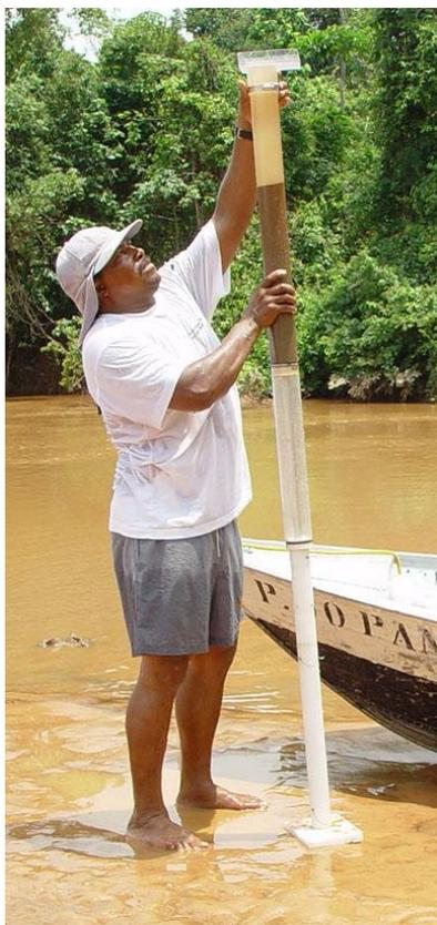
**Figura A2. Extrator de amostra “Core”.**
