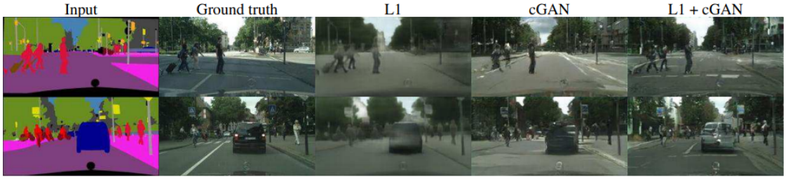
Figure 2.6: Different losses induce different quality of results in pix2pix. Each column shows results after being trained under a different loss by Isola et al. (2017).
