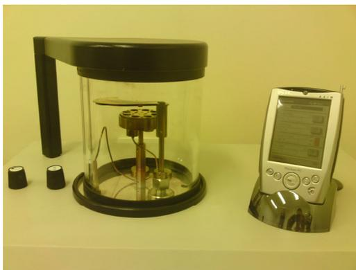
Figura 7 – evaporadora (*Sputter*) Denton Vacuum – Desk III<sup>®</sup>.
